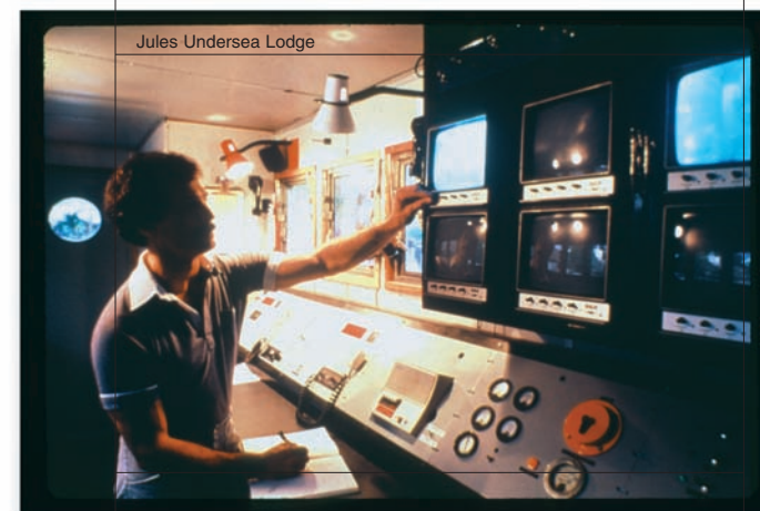
Main control van monitors life support systems for habitat from surface station. Communications are maintained by intercom, VHF radio and telephone
